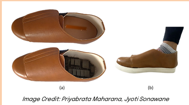
(a) Footwear with a self-offloading insole underneath the top sole (b) one of the volunteers wearing the self-offloading footwear
